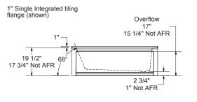
Wood support design may vary. Single Integrated tiling flange: 1" height x 1/4" thickness (shown) All dimensions are approximate. Structure measurements must be verified against the unit to ensure proper fit.
